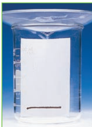
(a) Water-soluble ink is placed near the bottom of a piece of chromatography paper in shallow water.
