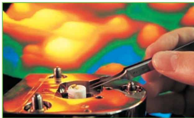
(b) A sample of DNA placed in a scanning tunneling microscope produces an image showing the contours of the DNA's surface.
