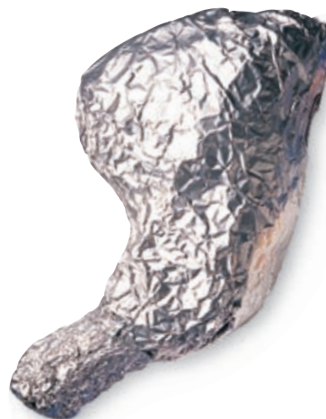
(c) Aluminum is malleable. It can be rolled into foil that is used for wrapping food.
