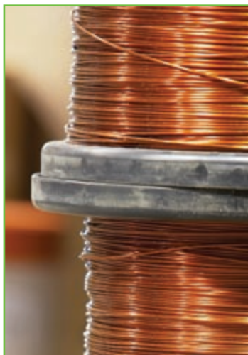
(b) Copper is used in wiring because it is ductile and conducts electrical energy.
